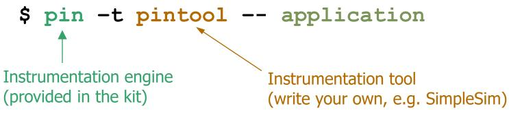
Attach to and instrument an application \$ pin -t pintool -pid 1234
