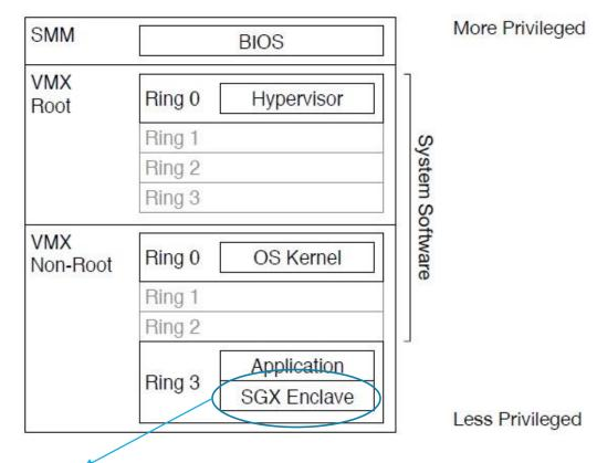
Part of Intel SGX: Secure execution of an application module.
